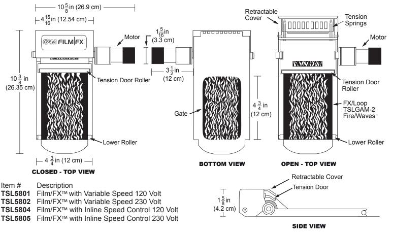
Film/FX<sup>™</sup> is supplied with attached transformer/power supply and can be plugged into any dimmer for speed control.
