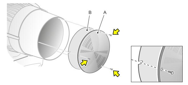
Figure 9. Removing a micro-Fresnel lens
