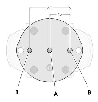
Figure 5. Mounting points in base
