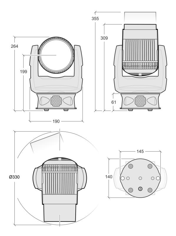
Dimensions given in millimeters
